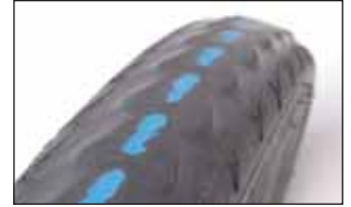
The puncture protection layer can be seen. The tire must be changed urgently.
