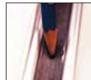
A rubber rim tape presses into the hole of a hollow section rim.
