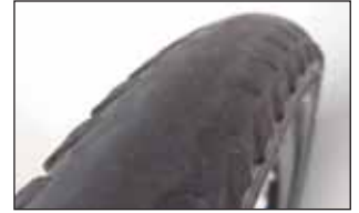
Tread is worn out. Rubber is still present. This tire can still be ridden.
