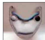
A wide tape that reaches from rim well to rim wall is a more secure solution.
