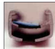
The rim tape is too narrow and does not cover the rim-well.
